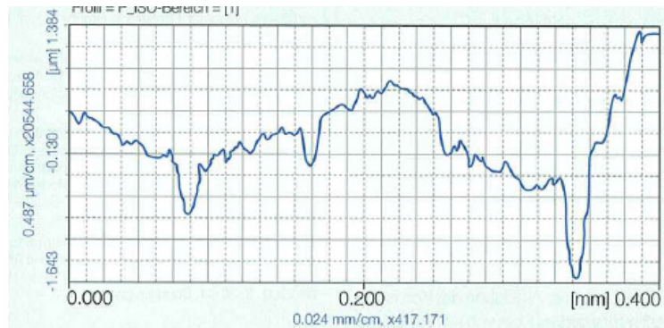
Fig. 6: Surface profile of a grain from the 1-2 mm fraction (a) and a glass bead 1.5 mm +/- 0.2 mm (b)
