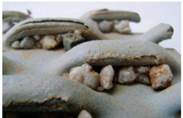
Often the well builder, as supplier of the well gravel, has difficulties and discussions with customers since the form of the individual gravel grains that are planned for the well construction cannot be described as spherical at all. It is apparent that the supplied gravel sometimes looks as though it has been broken, although this should not be the case according to DIN 4924.
