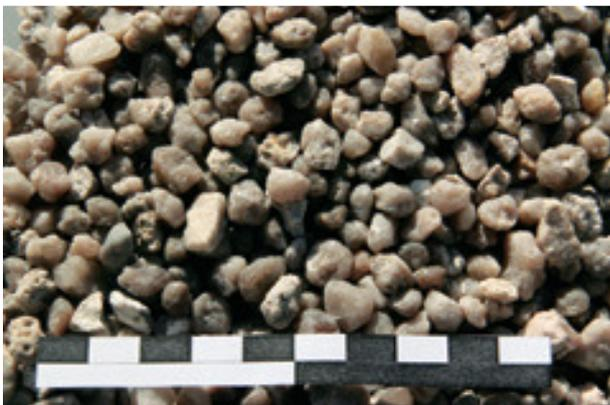
Sands and gravel, in accordance with DIN 4924, are unbroken natural quartz sand and gravel, without crimped or broken minerals. The requirements, in detail, are:
